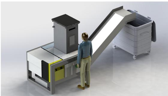
Automated file destruction system with briquetting press
